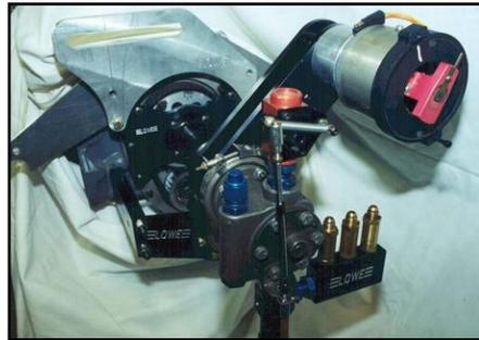
**it will sit outside the belt drive and allow you to rotate the offset drive clockwise or counter clockwise to give you the placement of the magneto that you want.**
