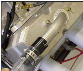
**Twist lock valve cover breather tubes, available in the old standard 2 bolt mount or the new 3 bolt mounting (shown).**
