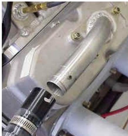
Quick Disconnect Valve cover vent tubes **3 bolt** hole mount 1 1/4" hose connection- 1/4 turn release with internal O-ring seal
