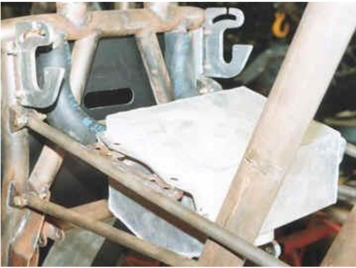
Puke tank on the back of an altered.
