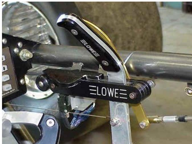
**Low gear** - Pulling the cockpit shift lever handle all the way to the back puts the transmission in low gear.
