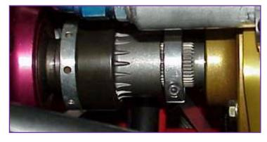
Complete Kit includes Powerglide adapter, coupler slide coupling and lock collar and does include the diff coupler
