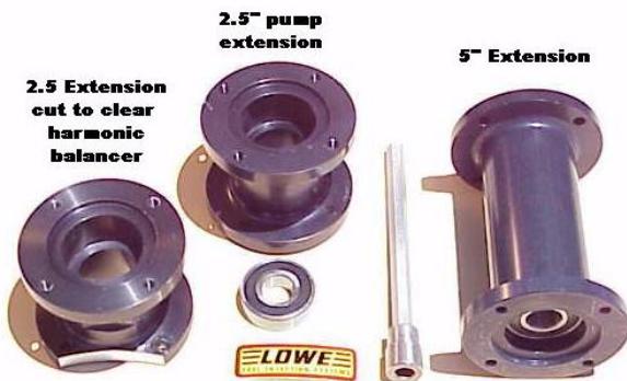
Extension assemblies include bearing and driveshaft
