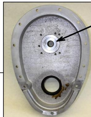
Removable cam thrust bushing. O-Ring seal around outside with lip seal for the cam drive to keep oil inside the engine without having to glue the pump to the timing case cover.
