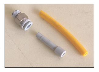
valve changing the fuel delivery at idle. Putting an "Idle Bleed Kit" in the hat below or after the butterflies allows you to adjust the air to the engine without having to adjust the butterflies. Usually three "Idle Bleed Kits" are all that is necessary to give you a full range of adjustment in air delivery at idle.
