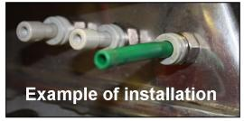
allowing max flow through this particular air bleed fitting. Can be used on both normally aspirated and supercharged engines.
