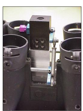
Having the barrel valve buried in the middle of the Crower Stack Injector makes it difficult to near impossible to adjust the idle volume or remove the hose connecting to the secondary check valve. Raising the barrel valve and extending the hex link makes access to these components easier to adjust.
