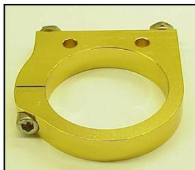
Bottle bracket to mount the 2" CO2 bottle in your car. Flat back mount allows mounting to any flat surface with two 1/4" unc bolts provided. One screw opens the bracket allowing the bottle to slide into place quickly and easily. Part number 84090-82000
