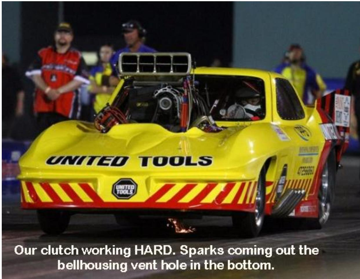
**Our clutch working HARD. Sparks coming out the bellhousing vent hole in the bottom.**
