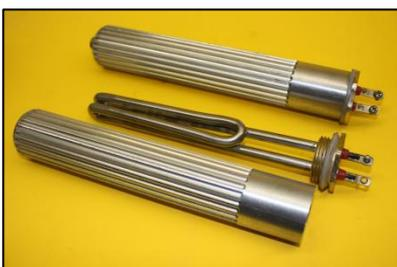
To increase the surface area ribs were cut into the aluminium housing increasing the surface area by 300%. Once assembled DOT5 brake fluid (270c boiling point) is put in to transfer the heat from the element to the body of the heater. One little trick is how to minimize the internal pressure build up when the DOT5 brake fluid is heated. After the units were assembled they were tested
