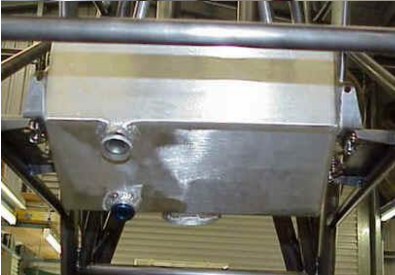
Puke tank on the back of an altered - see the sight gauge and the drain plug.
