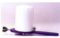
This aviation oil filter cutter will open any size oil filter canisters for your inspection. To use the tool, place the filter in a vice, attach the tool to the top of the filter, & rotate 4 to 6 turns to open the canister. Cutting wheel will stay sharp for about 50 uses, and is easily replaced when dull. The tool is made from 6061 aluminum anodized finish. The tool is ready to use on any oil filter with a male or female thread.
