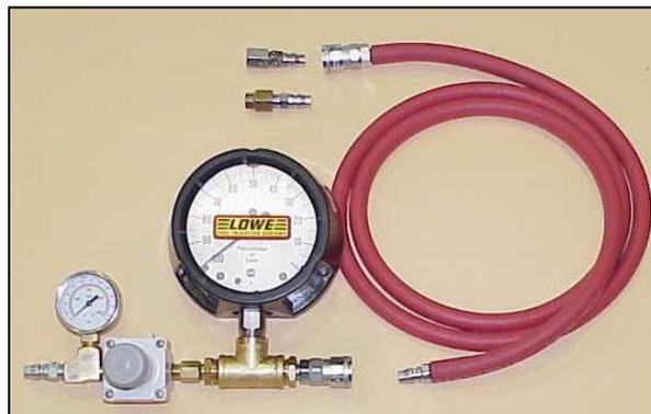
**Leak checker** Assembly includes calibrated (80% @ .080) leak checker with regulator, supply gauge, percentage of leak gauge, quick disconnects, and connector hose with quick disconnects from leak checker to accessory and calibration tool which can be used to flow check Enderle main jets. See below for accessories.
