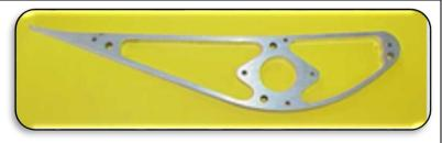
Here is how the billet wing spar fits into the end of the wing. The billet spar is used to hold the end of the wing and the spill plates together.
