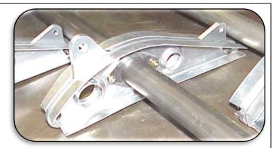
The billet wing spar and the support bar flange are bolted together and then TIG welded to the center support bar to create an extremely robust structure to mount the skin to.
