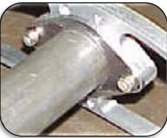
This photo shows the formed spars attached to the billet aluminum mounting plate with the center support bar flange in place and the chrom moly center support bar in place to make the wing near "shake proof". The support bar flange gets TIG welded to the support bar before the skinning begins.
