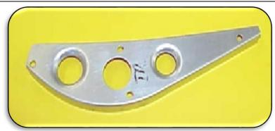
View from the other side, this is a right throw flanged formed wing spar. A pair of left and right make a pair of formed wing spars for a very light but very strong wing.
