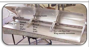
Skin material is standard 0.8mm thick or polished 0.5mm with plastic coating (shown).
