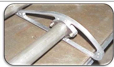
Once all the spars are TIG welded to the center support bar you are ready for skinning. Form the aluminum skin over the spars and rivet in place.
